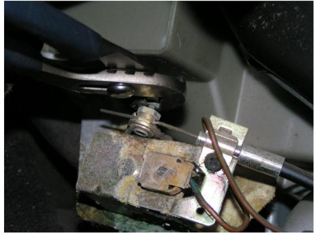
Use a screwdriver to loosen the cable clamp. Remove the clamp completely.
