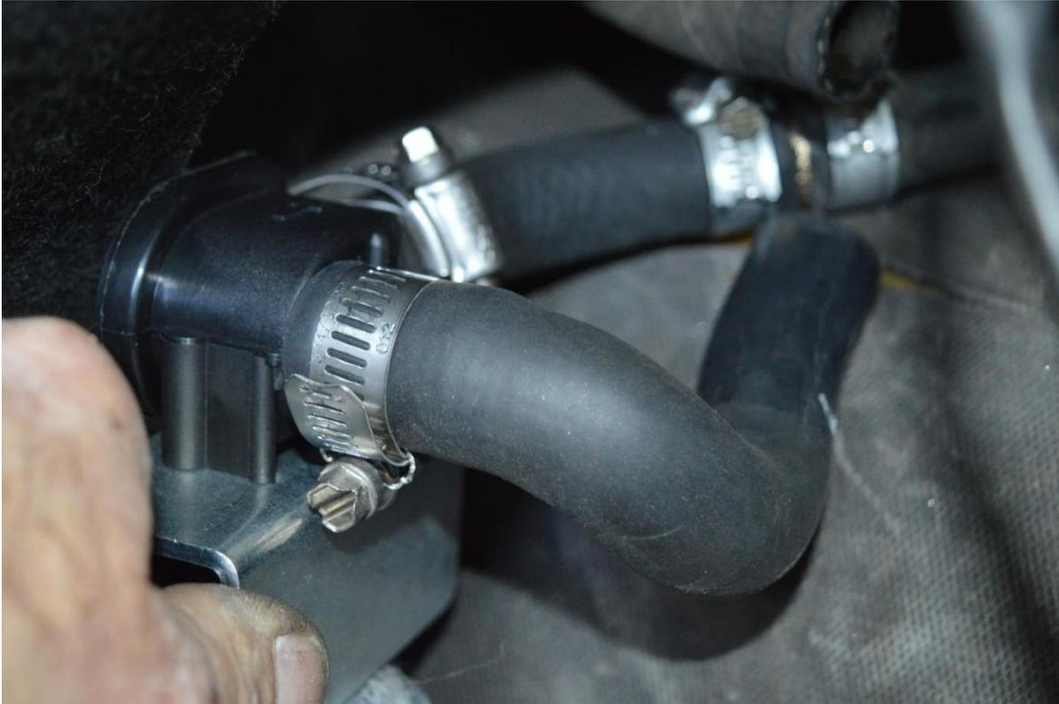
Rotate the valve around and install the second hose splice for the inlet hose. Pay attention to orientation of hose clamps or something will rub or hit another hose—or the valve's actuator arm.
