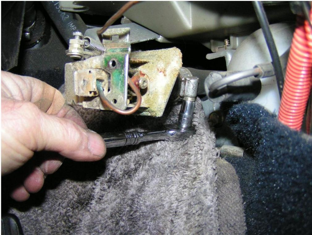
The hoses will be stuck tightly to the valve! Be careful. If you tear them, they will have to be replaced. Work a small screwdriver under the edges of the hoses to help loosen them. The old valve will likely be somewhat corroded, depending on how much humidity has been present. This one was not too bad—a desert car.
