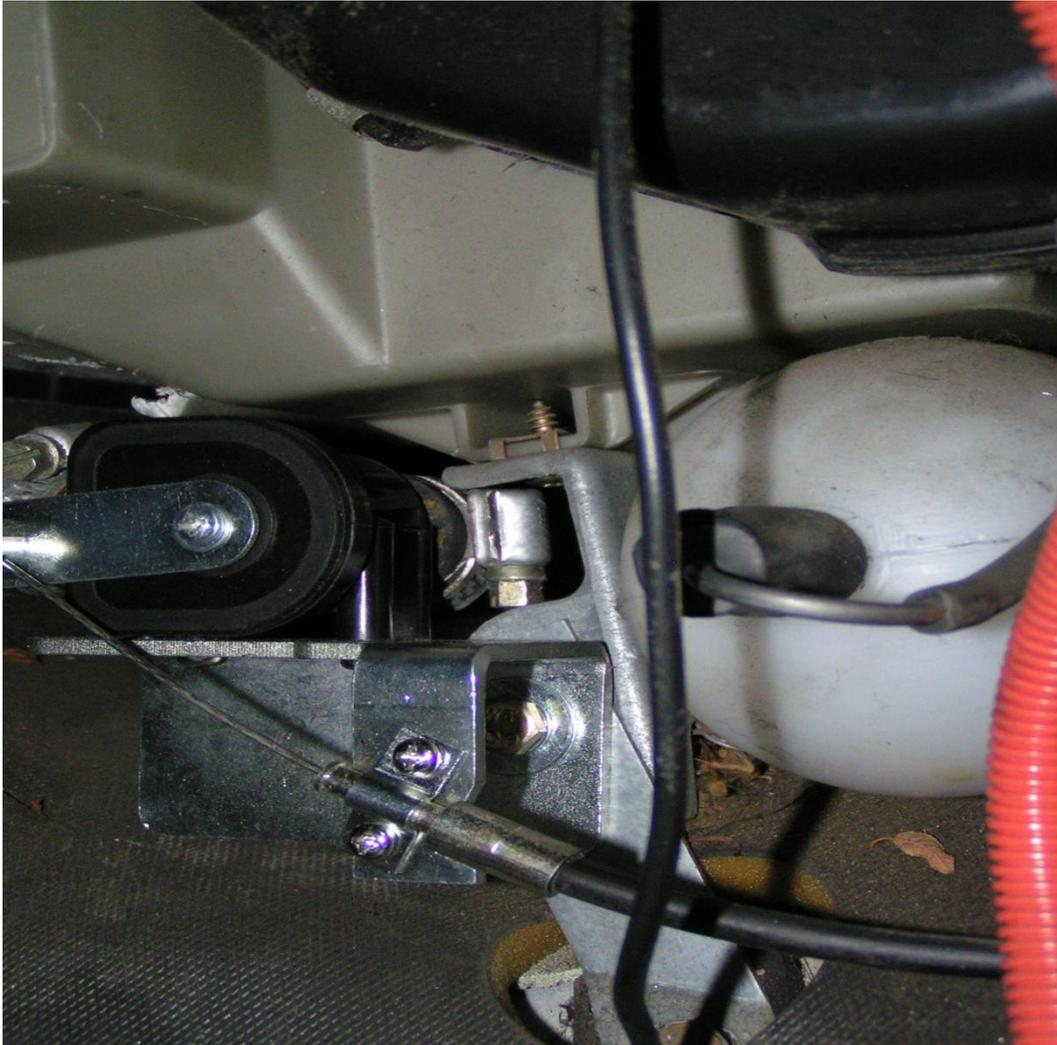
If you feel you pushed a lot of the passenger side (outlet) hose back in behind the heater box, it is wise to check under the right side of the dash and make sure the hose is not rubbing against the windshield wiper linkage. The hose may have worked its way upward when you pushed it back in place. If so, arrange the hose to clear the linkage and consider fixing it in place to the AC plumbing if it will not stay put.
