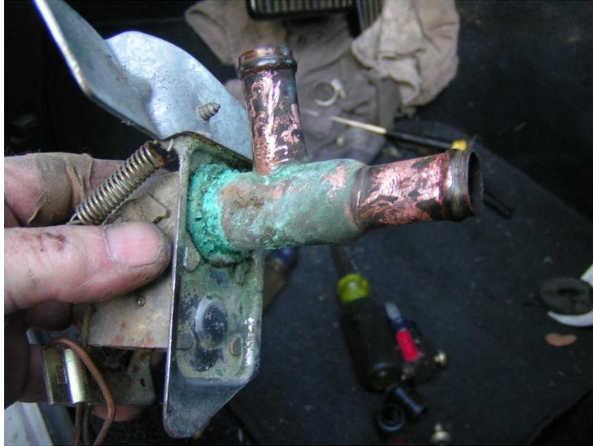
With the heater valve pulled down, remove the capillary tube assembly from the heater box. You will need to pull out the oval rubber grommet too. Here you can see the capillary tube assembly exiting the bottom of the blower motor scroll housing.
