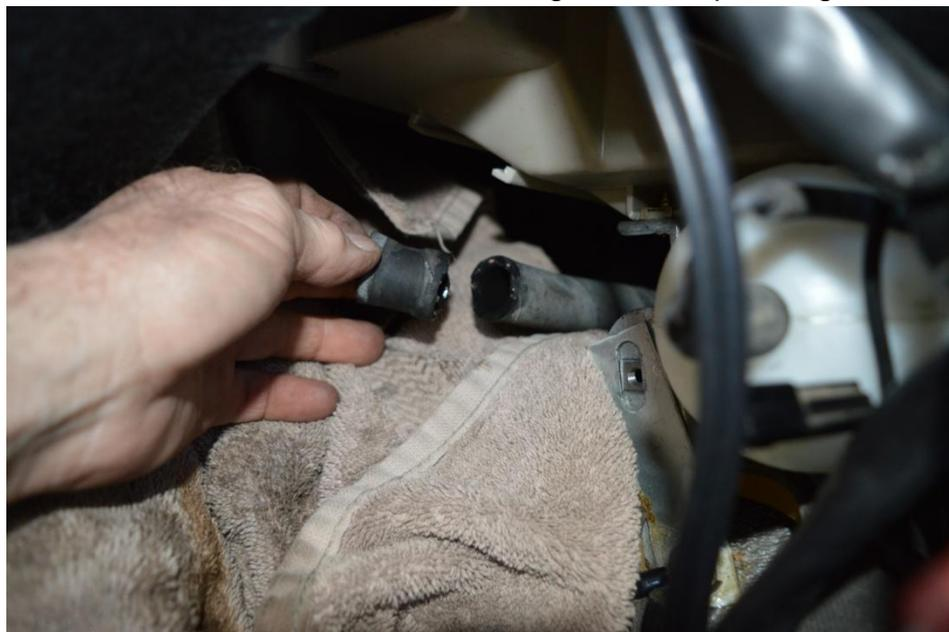
Insert one of the hose splices and secure with a hose clamp.
