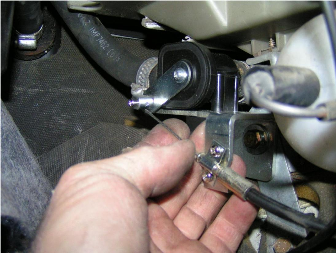
Adjust the wire in the swivel and also the cable in the attachment clamp so that when the heater control lever is off, the valve is fully closed—arm in the up position. You must use almost all the length of the cable to assure the heater control lever on the dashboard moves the valve's arm all the way to "closed". If the valve stays open, your air conditioning will not function correctly.
