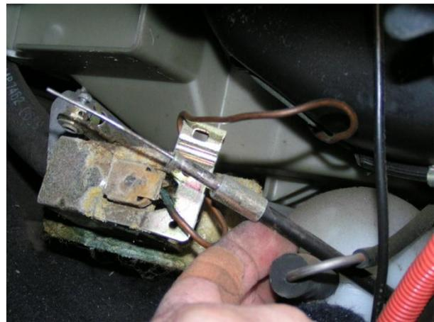
Reposition the cable below any vacuum plumbing for the HVAC vacuum canister.
