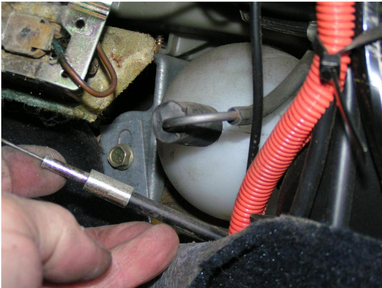
Grasp the old valve firmly and pull the top bracket out of the back of the heater box.
